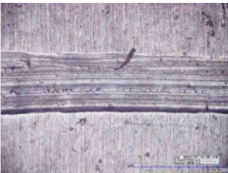
Figure 3. Intermediate fault in outer race.
