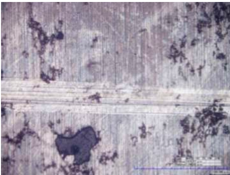
Figure 2. Incipient fault in outer race.
