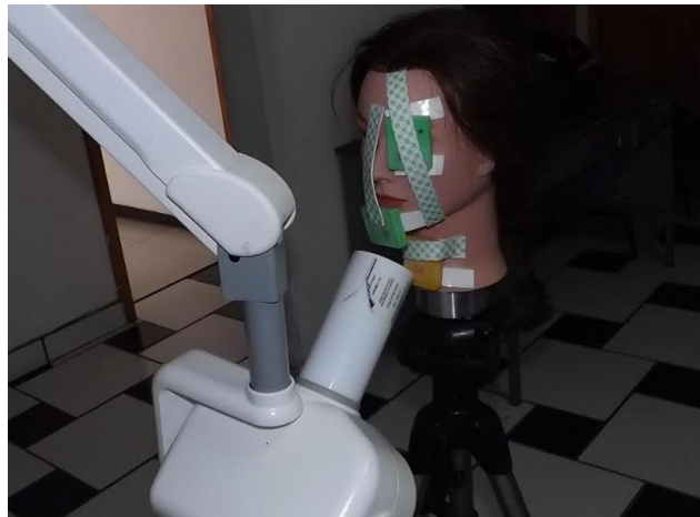
Fig. 1. B Patient phantom with the TLDs being exposed to dental X-rays (Frontal Exposure).
