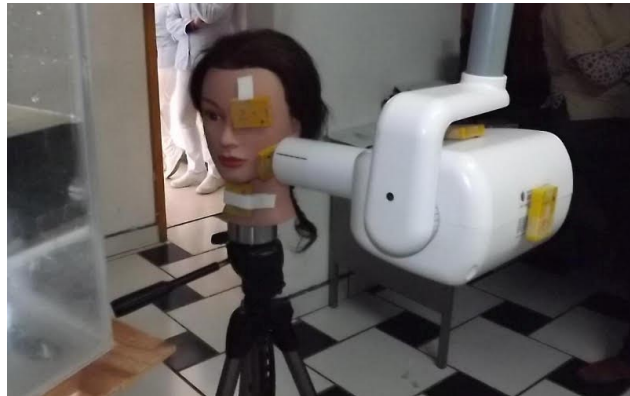
Fig. 1. A Patient phantom with the TLDs being exposed to dental X-rays (Side Exposure).
