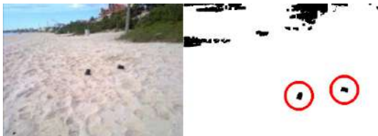
Figure 15. Image obtained by the camera (left) and the two black cans detected by the algorithm (right).
