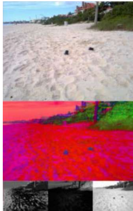
Figure 5. Camera image (top), converted to HSV (middle) and each HSV channel separately (bottom).
