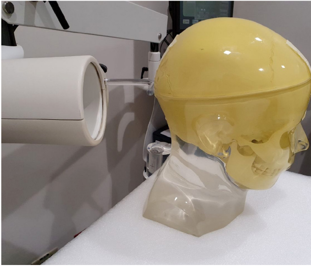
Figure 2. Head geometry for the calibration of 18 F-FDG in vivo measurements.
