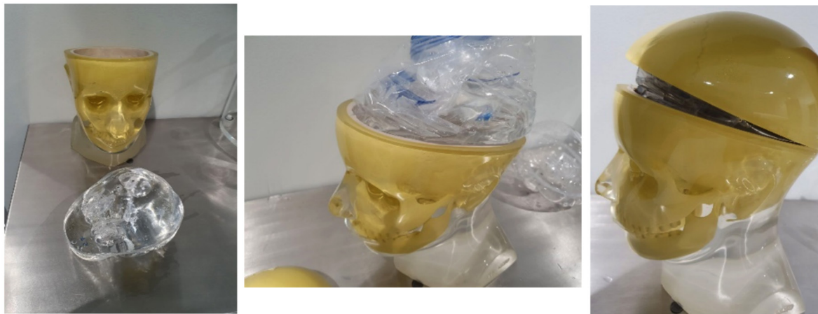
Figure 1. Head phantom assembly for calibration. a) Filling of the brain accessory with water. b) Transfer of the water volume from the brain accessory to a plastic bag and placement of the calibration source. c) Assembly of the head phantom.
