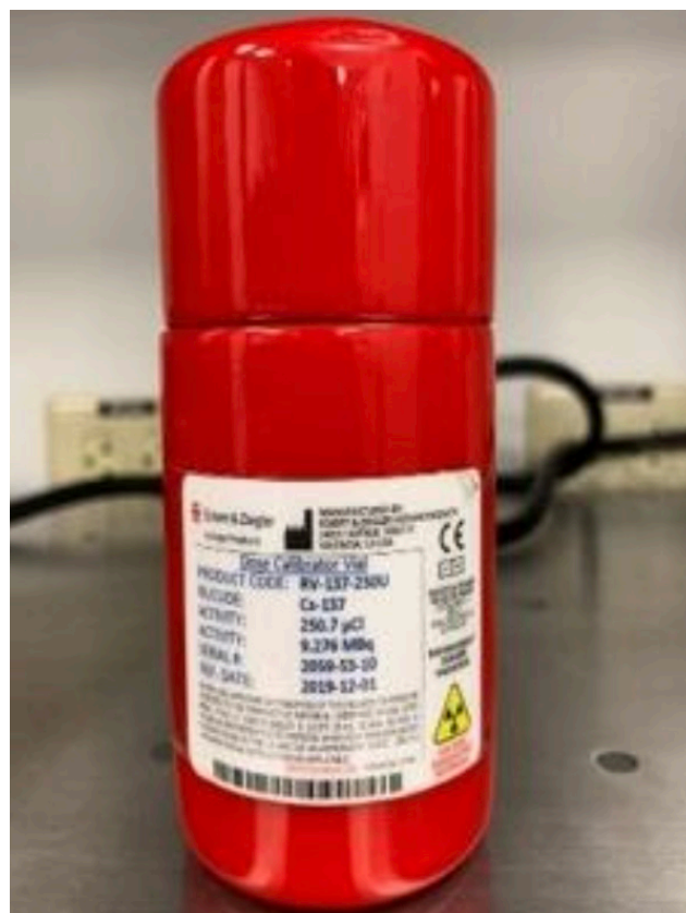
Fig. 1. ^{137}\text{Cs} radioactive source used to perform all of the measurements for the characterization done in this study inside its lead case.
