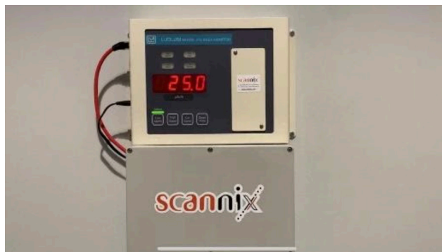
Fig. 3. Display of the Geiger-Müller sensor located outside its respective room showing the current reading of radiation exposure.
