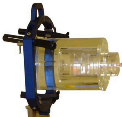
Fig. 1. Head phantom mounted in a Lecksell-type frame with its various components used for performing the tests.
