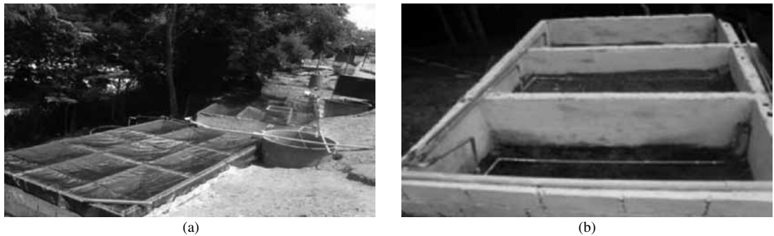
Figure 1. Experimental apparatus with 27 cement biofilters (a); detail of the biofilters (b).
